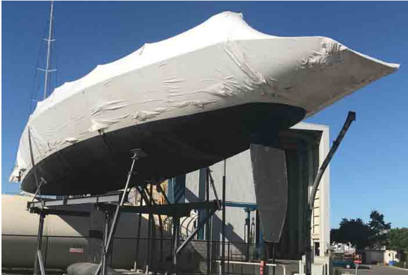
Narrow water line of ex AC hulls makes an ideal conversion to a power trimaran
