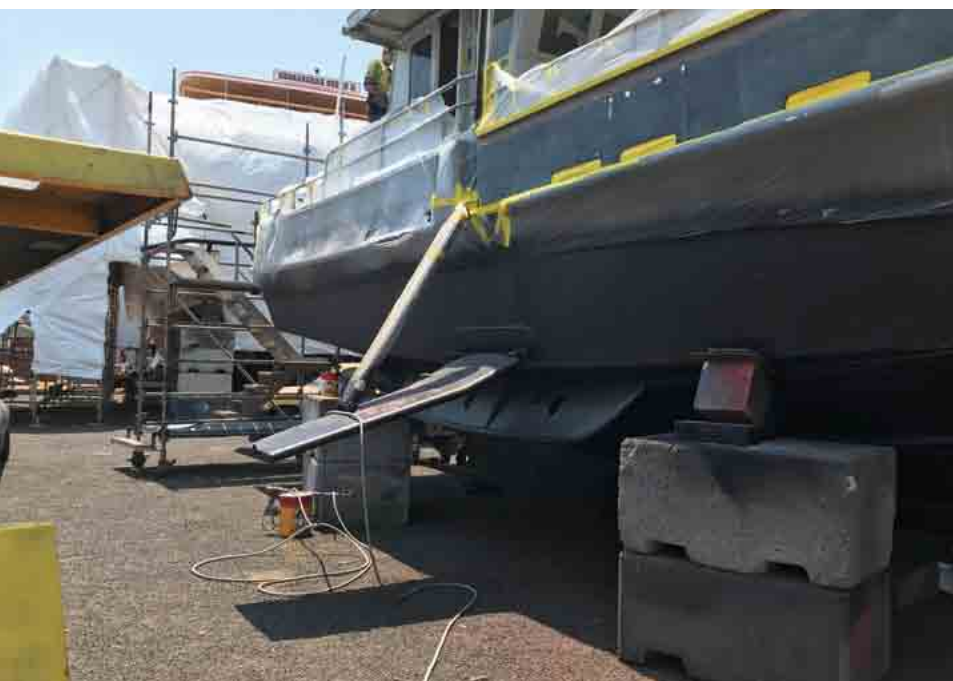
TOP: Stabiliser foils fold up when not in use on another fishing boat to reduce drag.
