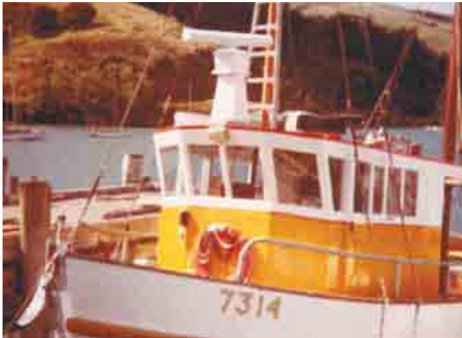
Jean composite panel wheelhouse finished with first bonded in windows.
