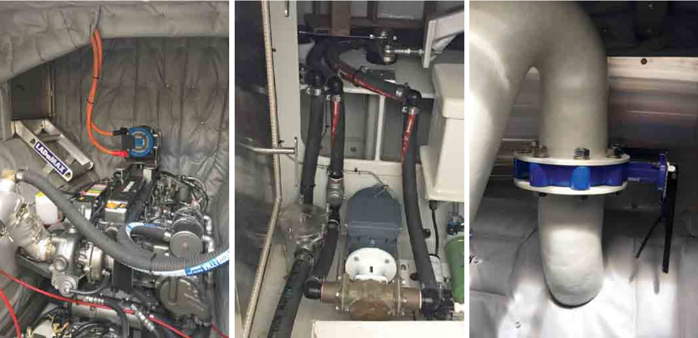
ABOVE LEFT: Engineroom with rough water access, custom fire cladding and military spec alternator mounted on custom frame bolted to engine.
