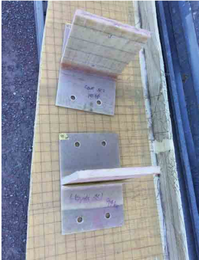
Tests comparing a standard Lloyds tabbed bulkhead join with a Crestomer 1152PA coved join demonstate that the coved join is over twice as strong
