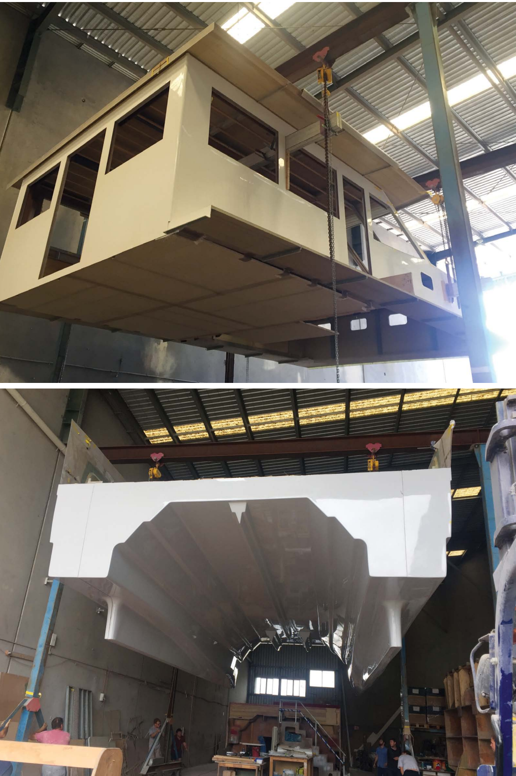
TOP: The cabin, side decks and saloon floor being lifted into position. ABOVE: The hull being lifted out of the mould by the bulkheads with their new bonding system then moved into the other shed.
