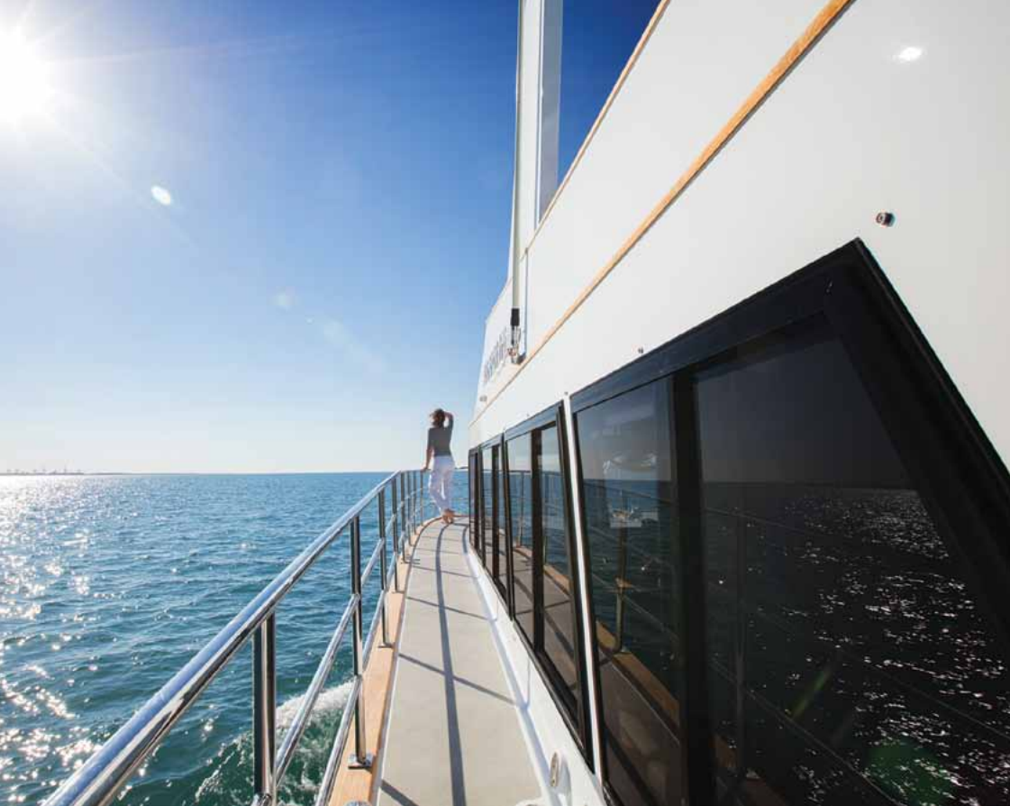
ABOVE: Sliding windows on both sides of the cabin for visibility and ventilation.
